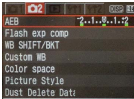
Canon Rebel XT/400D LCD showing AEB with +/-2 increments selected
