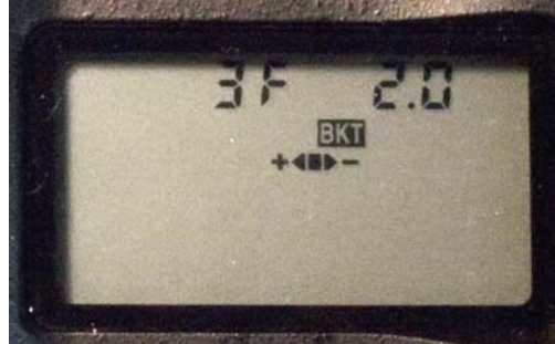
AEB settings at the top of the LCD of a Nikon D80 (3 shots with +/- 2EV)
